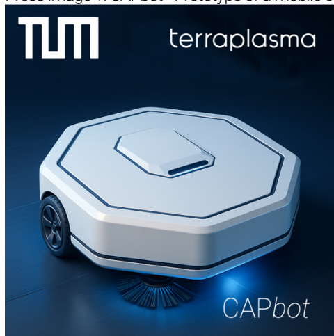
Press image 1: CAPbot - Prototype of a mobile cleaning robot with plasma-activated fog
